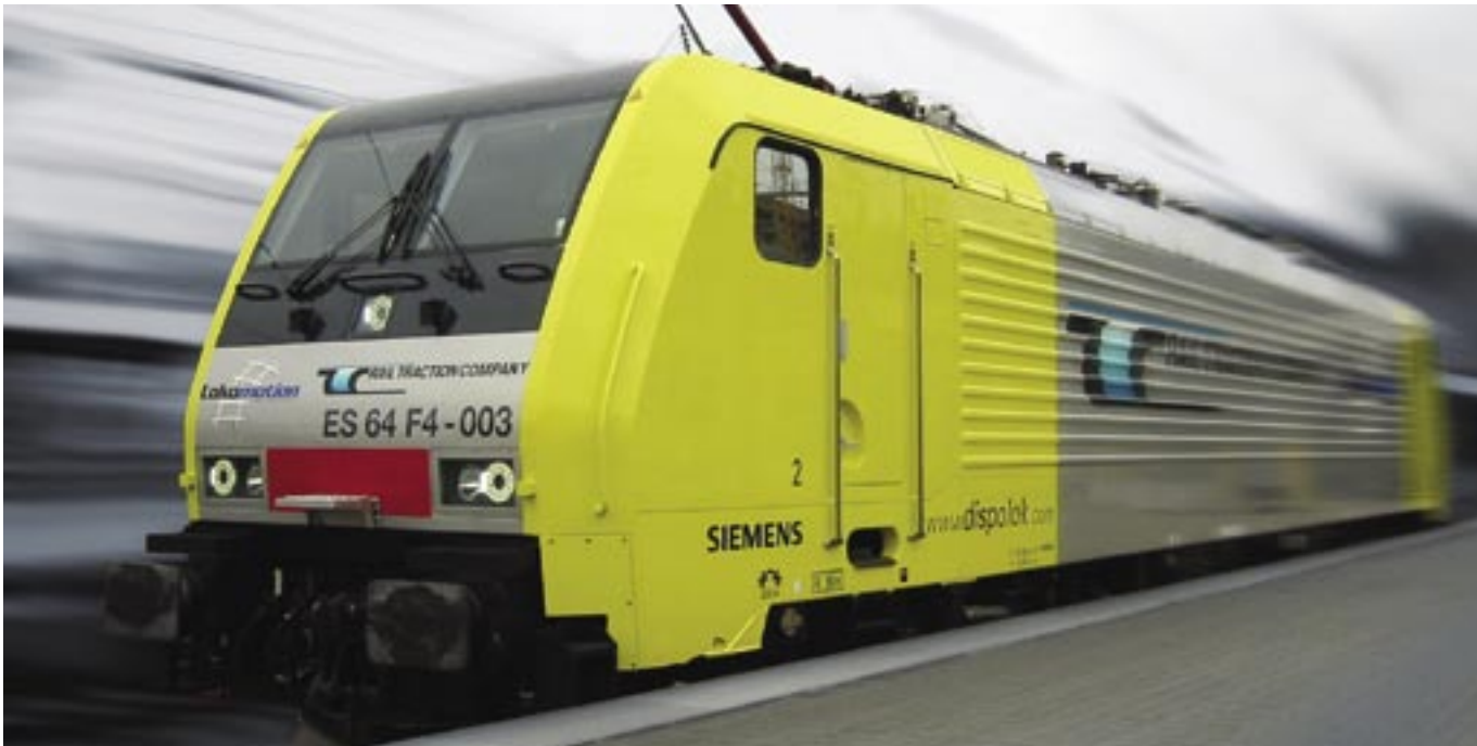
The EuroSprinter ES 64 F4 locomotive is able to operate at all common voltages used in Europe and is thus ideal for cross-border rail traffic.
