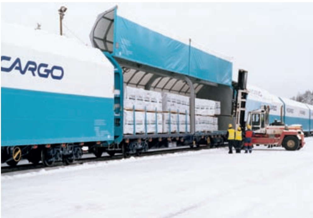
VR Cargo designs wagons with its customers. Shown here, a new wagon for sawn timber with a two-section roof that withstands strong winds.
