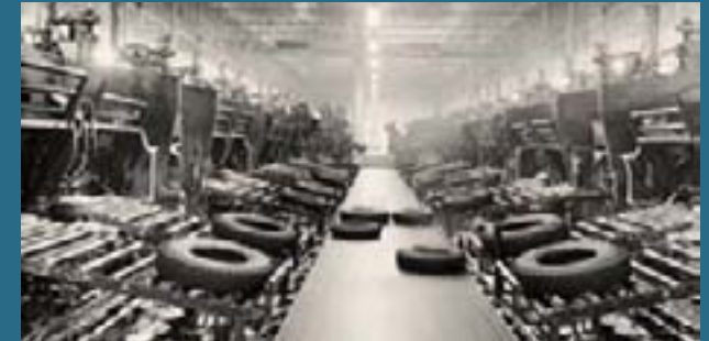
A curing hall in the 1970's: The Hakkapeliitta tyres go from curing moulds to the conveyor belt.
