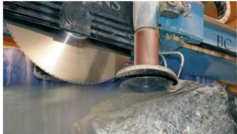
1. The block cutter that was introduced at the custom-made plant in the year now ended boosts the efficiency of soapstone processing.
