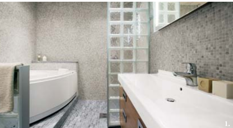
1. Soapstone mosaic tiles with a brick pattern liven up the floor. Soapstone is very suitable for moist areas, because it is not slippery when wet and retains heat well. On the walls: Cloudy Grey marble mosaic tiles.
