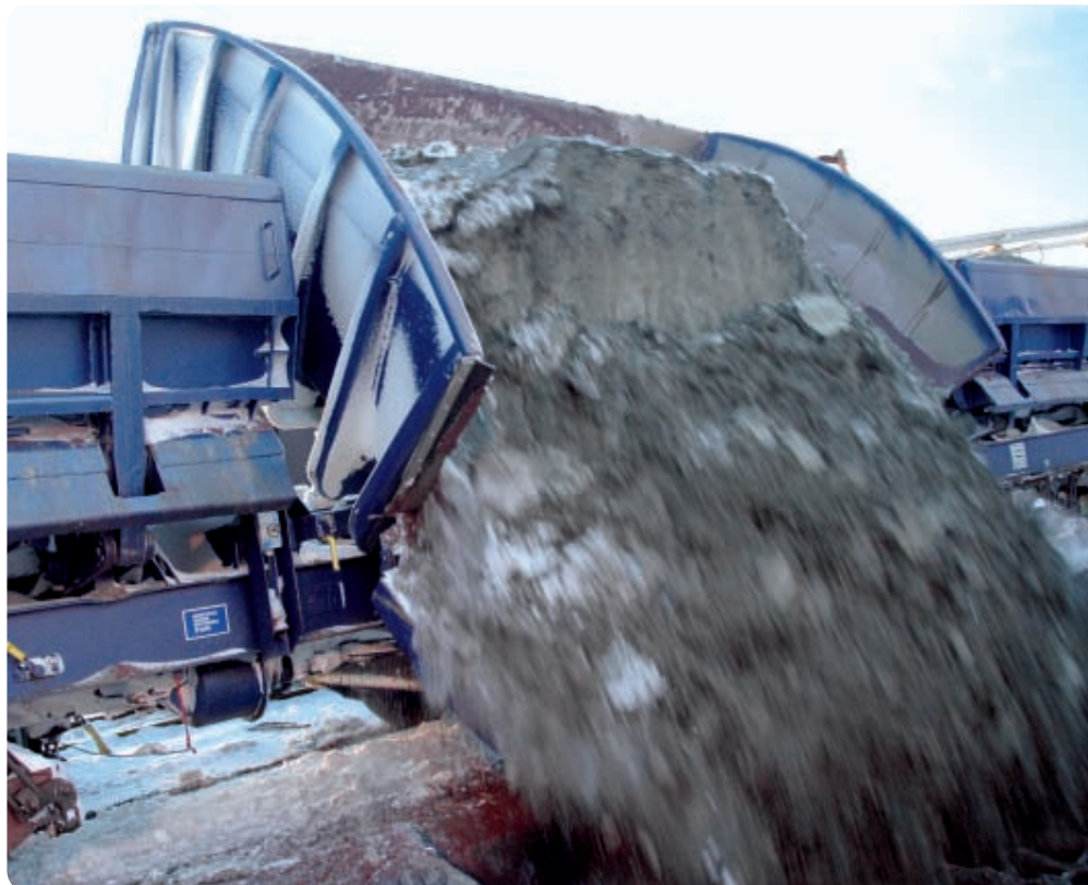
VR's goal is to plan transport systems that best meet customer needs. Part of these projects involves developing rolling stock. The picture shows the new version of the ore-carrying wagons used for transporting ore concentrates.
