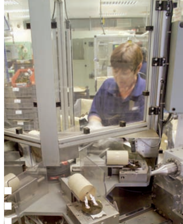
■ Ultrasonic welding and rivetting of electrode contacts at BHC Component's factory.
