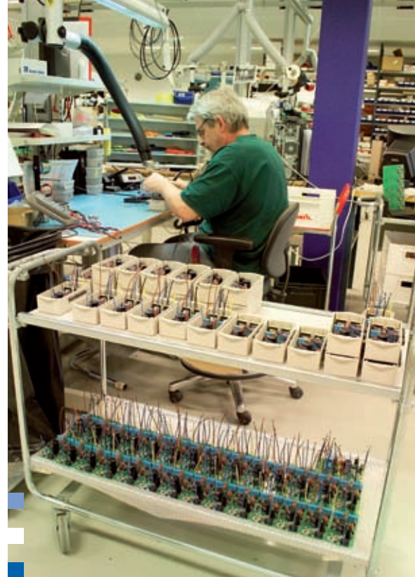
Customised EMI suppression filter production utilising Evox Rifa capacitors in Dectron AB.
