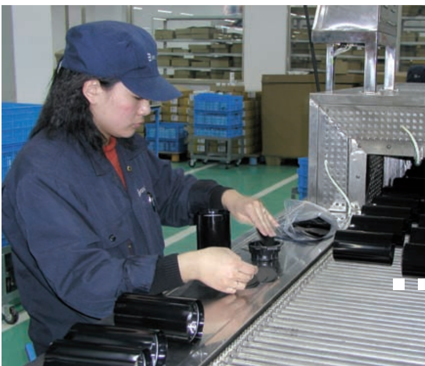
■ ■ ■ ■ ■ Applying insulating sleeves on capacitors at Evox Rifa's Nantong factory.
