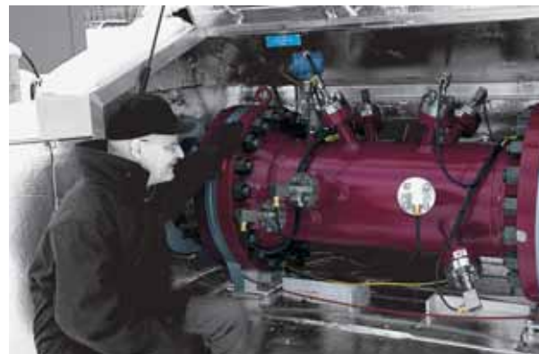
Control room technician Heimo Komi checks the operation of an ultrasonic flow meter in test use.
