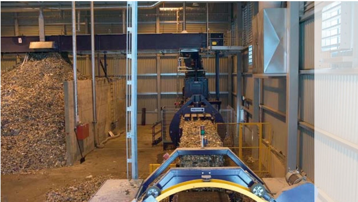
L&T collects burnable waste and processes it into recovered fuel for power plants.
