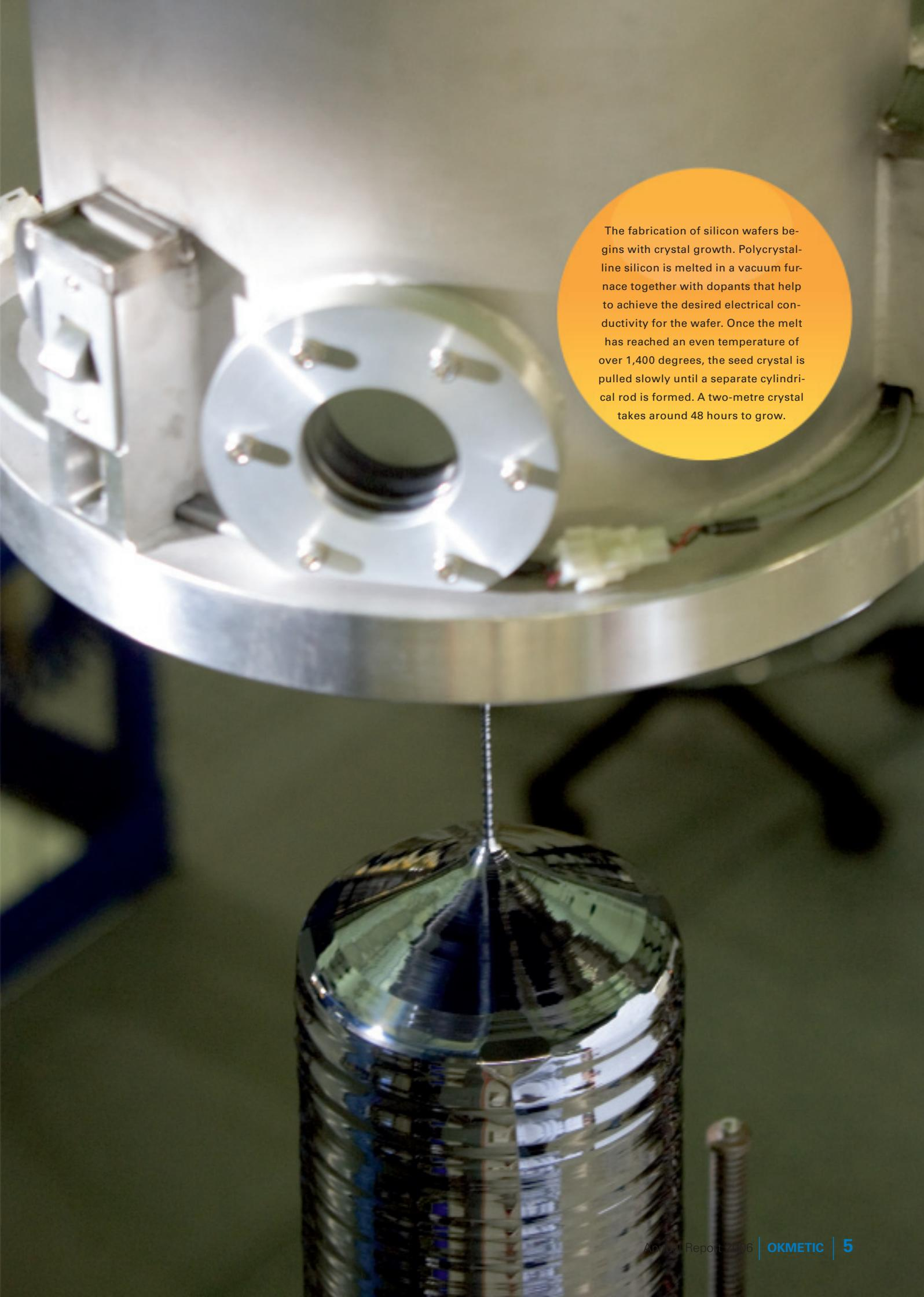
The fabrication of silicon wafers begins with crystal growth. Polycrystalline silicon is melted in a vacuum furnace together with dopants that help to achieve the desired electrical conductivity for the wafer. Once the melt has reached an even temperature of over 1,400 degrees, the seed crystal is pulled slowly until a separate cylindrical rod is formed. A two-metre crystal takes around 48 hours to grow.
