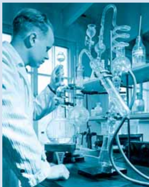
Mr. O. Erik Virtanen producing penicillin at Orion in 1945. The neutralised penicillin concentration was frozen, and the frozen water was removed under a low pressure achieved by the help of a diffusion pump.
